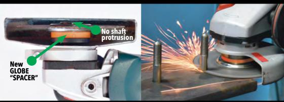
Thanks to the use of the special **"SPACER"** and to the depressed center shape, the machine shaft and the locknut do not extend from the dome cavity thus enabling the operator to carry out flush cuts in a comfortable and safe position. The depressed center shape gives more rigidity than a flat disc, prevents bending allowing to make perfectly straight cuts.
